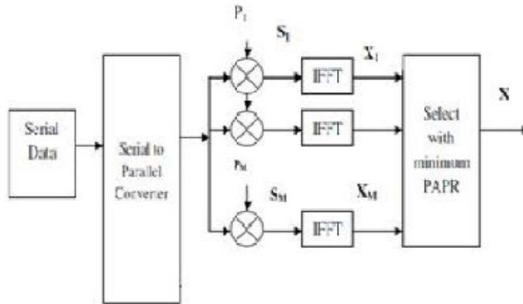
Figure 3: OFDM Transmitter Section With SLM Scheme
