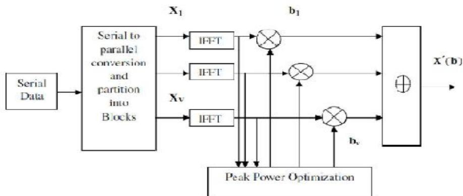
Figure 4: OFDM Transmitter Section With PTS Scheme
