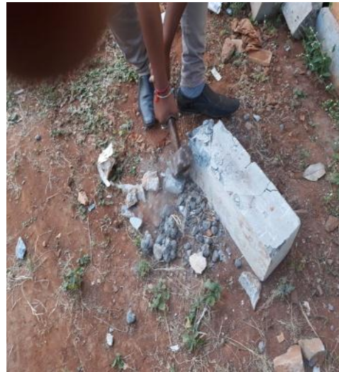
Fig 2: Separation Of RCA From Cubes
