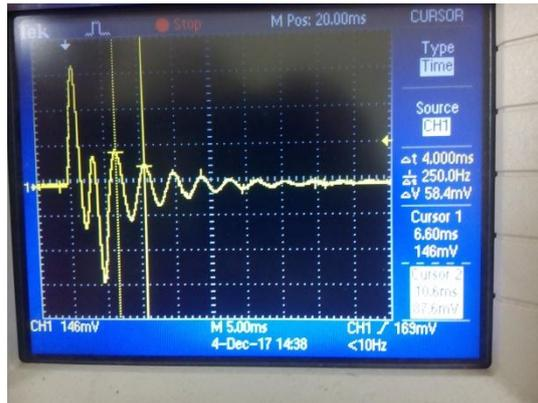
Figure 6. Acoustic resonance frequency of speaker
