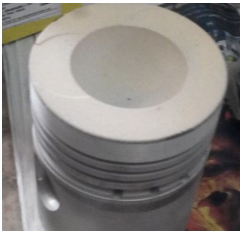
Fig. 4. Yitriya stabilized Zirconia coated piston
