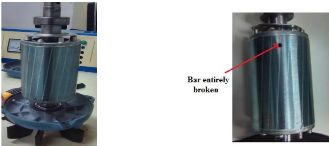
(a) Healthy rotor (without defect)
