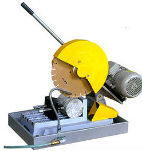
Figure1. Equipment for Slicing of Concrete Cylinders into Discs
