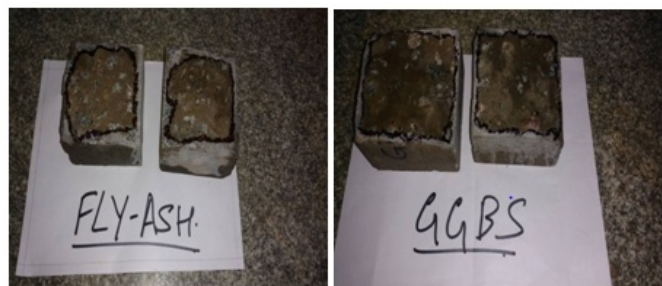
Figure3. Typical Cut Concrete Specimens after 28 Days of Immersion
