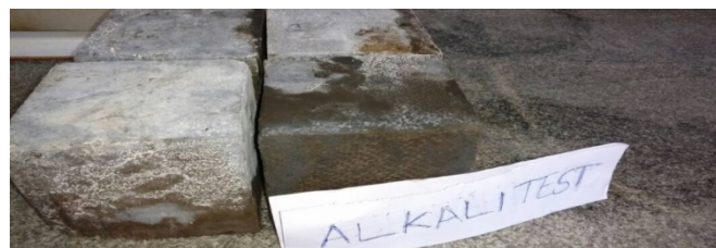
Figure 6. 28 days Alkaline cured concrete specimens
