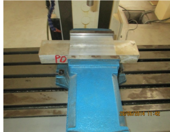
Fig 2.2 clamping of work piece on milling machine
