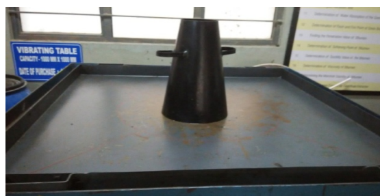
Fig. 5 slump flow Apparatus
