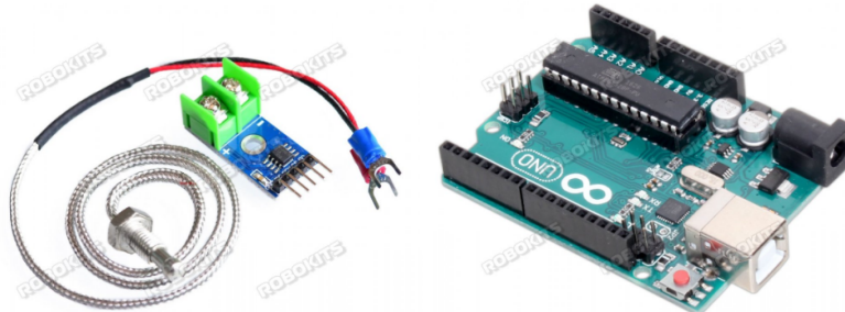
Fig.3. Arduino UNO R3 board and MAX 6675 temperature sensor with K type thermocouple
