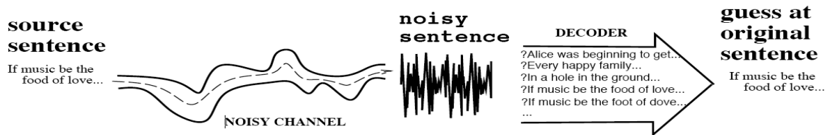
Figure 1: The Noisy-Channel Model 1
