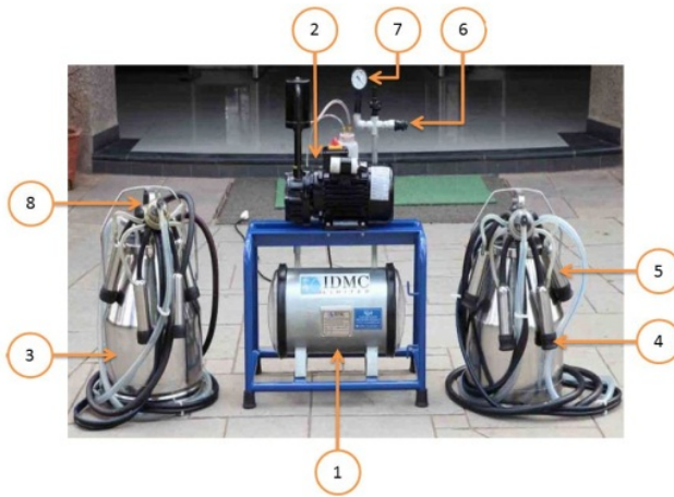
Figure2. Fix Type Milking Machine
