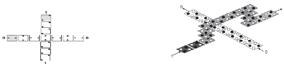
Fig 7: (a) Coplanar Crossover (b) Multilayer Crossover
