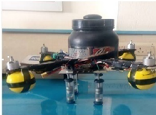
Figure 5: Magnetic shock absorber landing
