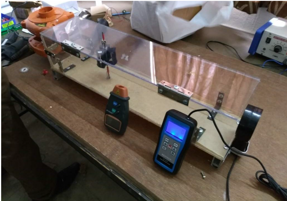
Fig. 5: Testing of Micro-Darrius vertical axis wind turbin
