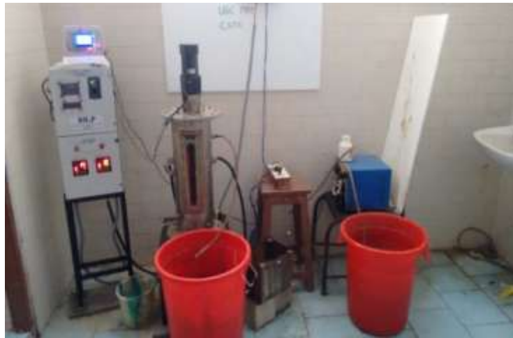
Fig. 2 Real Set up of Continuous Flow Stirred Tank Reactor
