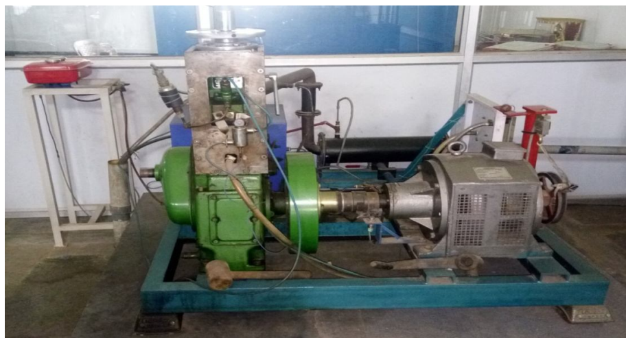
Plate 2: diesel engine test rig
