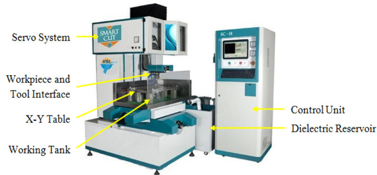
Figure 2: Experimental setup of Wire EDM
