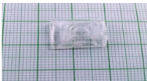
Figure 1. Succinic acid doped ADP crystal
