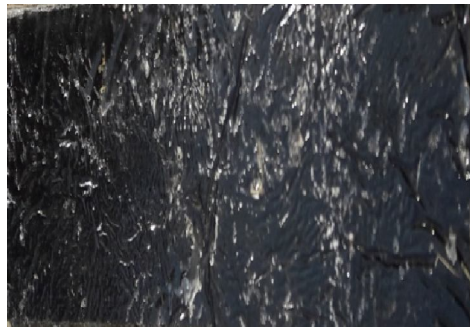
Fig 5: Human hair-20%, sheep hair – 10% Bamboo fiber- 10 %, Epoxy – 60%
