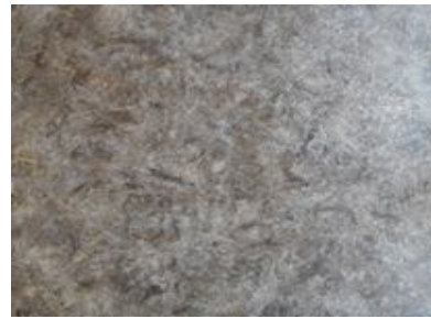
Fig 4: Human hair-10%, sheep hair-10%, Bamboo fiber-20 Bamboo fiber-10 %, Epoxy-60%
