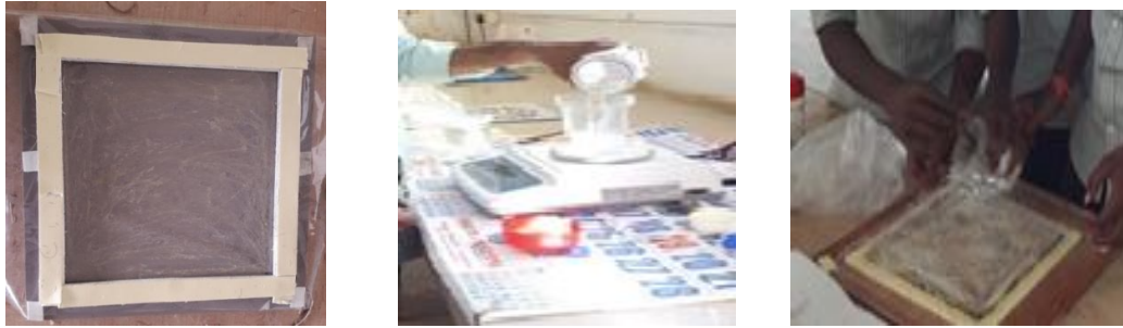
Fig 2: Preparation of mould, weighing & applying epoxy for hybrid composite
