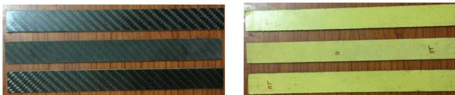
Figure2. Specimen Used for Tensile Test
