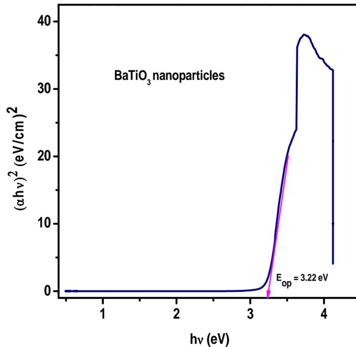
5. The  $\alpha h\nu$  versus photon energy of BT nanoparticles.
