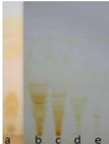
Fig. 1: Retardation factor of bio-oils, a- Standard Jatropha oil, b- Pongamia oil, c- Used Sunflower oil, d- Neem oil, e- Palm oil
