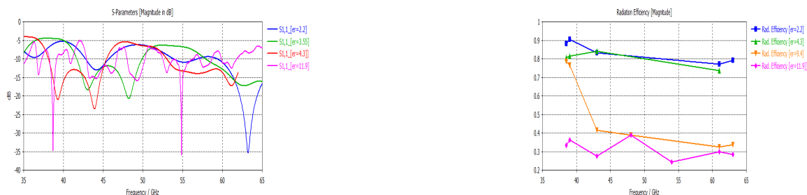
Figure 6 Effect of Substrate Dielectric Constant on Return Loss and Radiation Efficiency
