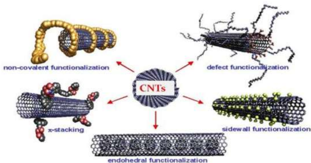
Figure 4: Methods of functionalization of carbon nanotubes
