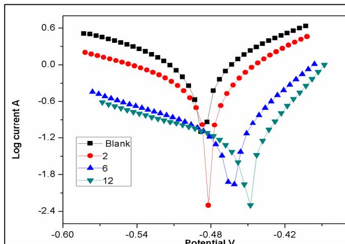
Fig. 7 Polarisation curves showing influence of increasing concentrations of *R. damascena* leaves extract on mild steel in 0.5 M H<sub>2</sub>SO<sub>4</sub>
