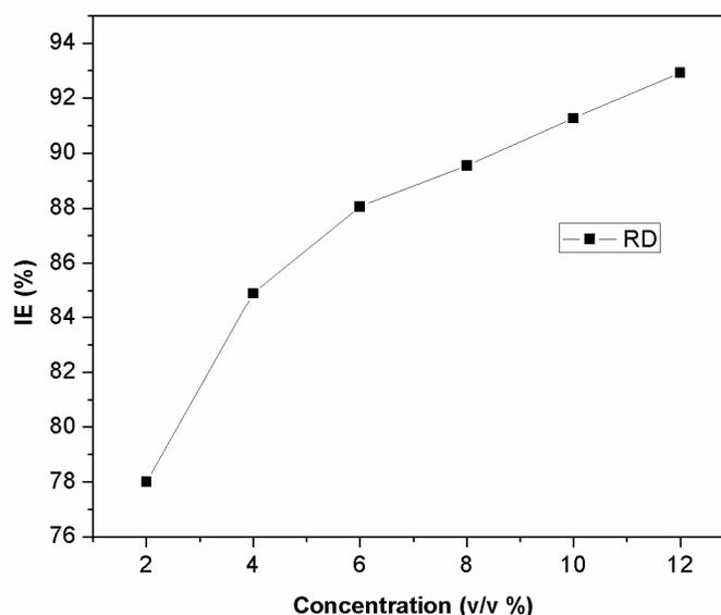
**Fig. 1 Variation of inhibition efficiency with concentration on mild steel in 0.5M H<sub>2</sub>SO<sub>4</sub> in presence of *R. damascena***
