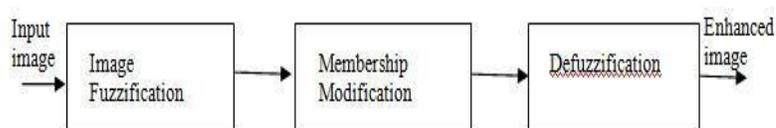
Figure 1. The main principle of Fuzzy Image enhancement
