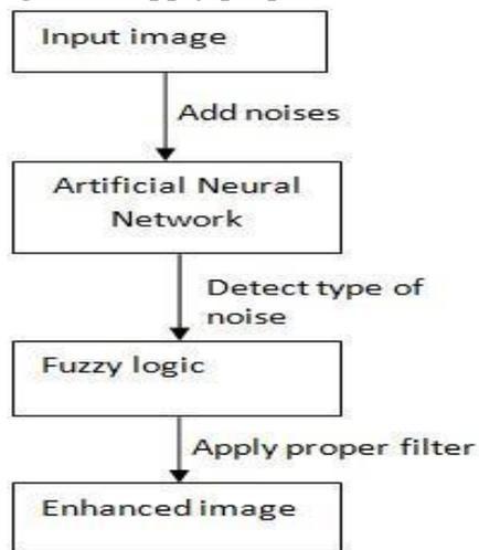
Figure 2. The principle of Nuro-Fuzzy Image enhancement
