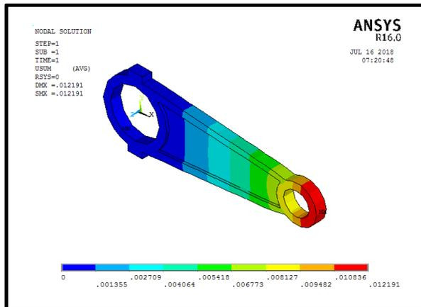
Fig11. Displacement Plot of MMC1 (3% Fly ash and 3% SiC)
