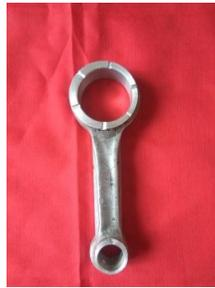
Fig 5. Finished connecting rod squeeze casted composite
