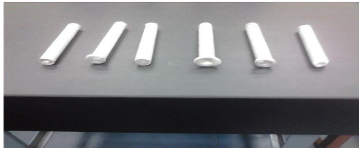
**Fig3. Squeeze casted composites**
