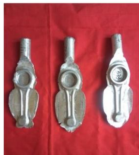
**Fig 4. Semi-finished connecting rod squeeze casted composites**
