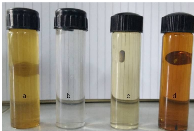
Fig.1 Green synthesis of AgNPs (a) Plant extract (b) Silver nitrate solution (c) 1mM silver nitrate + plant extract at the start of incubation (d) S. tumbuggaia AgNPs
