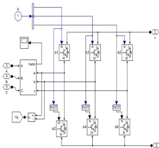
Fig (2) Switching operation of Series Filter Controller
