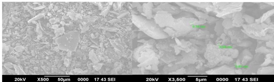
**Fig 2: Scanning Electron Micrograph of powdered rice husk.**
