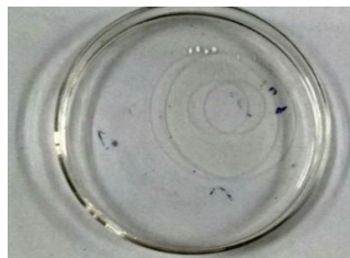
1: Demonstration of Oil Spreading by Biosurfactant
