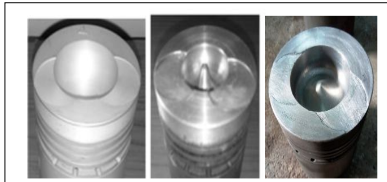
Figure 2 Different types of pistons shown in the above figure, like Hemispherical, Toroidal and shallow depth shapes to test biodiesel
