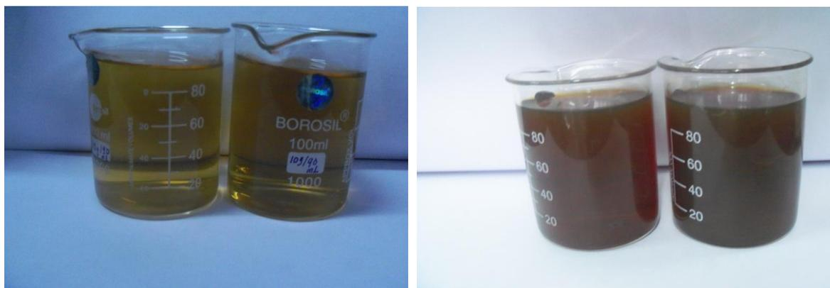
Fig 1. Photographs showing colour changes after adding chitosan- curcumin before reaction (a) and after reaction time of 10-12 h.
