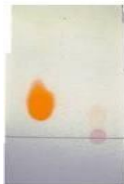
Figure 7. Identification Acid orange 10 dye degraded product on TLC (Rf values of control dye and decolorized sample).
