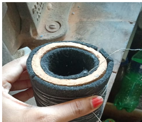
Figure 4 Electrodes wound around the membrane
