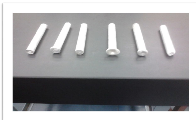
Fig. 3 Squeeze cast composites after removing from the molds
