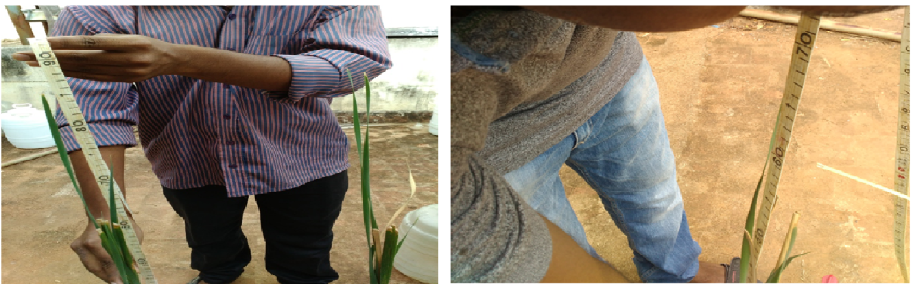
Figure -17: Measuring heights of TyphaAngustifolia in wetland model and in blank under Hydric Soil Substrate The initial height of TyphaAngustifolia is 60 centimeter. Average height of TyphaAngustifolia in the model is 88 centimeter against 63 centimeter in the blank, possibly due to nutrient uptake from supplied wastewater at the end of all discharges.
