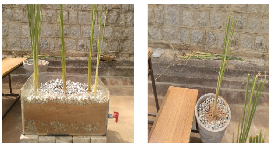
Figure -4: VSSFCW (model and blank) with Typha Angustifolia in Sandy loam soil substrate
