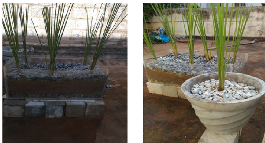
Figure -3: VSSFCW (model and blank) with Typha Angustifolia in Hydric soil substrate
