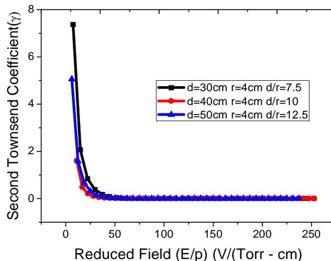
Figure 11: Variation of second Townsend coefficient ( $\gamma$ ) as a function of  $E/p$  for different distances
