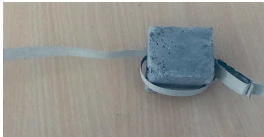
Figure3. Block at the end of the reinforcement
