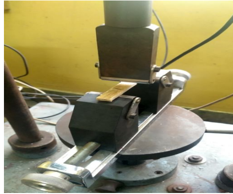
Fig 9: Flexural test equipment
