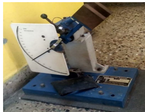
Fig 8: Izod test equipment
