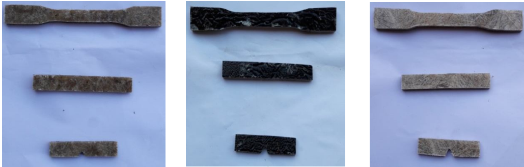
Fig6: ASTM standard specimens for testing
