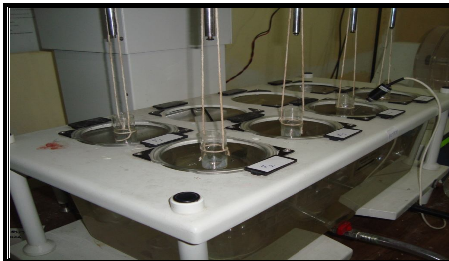
Figure 4 Modified USP dissolution test apparatus.
