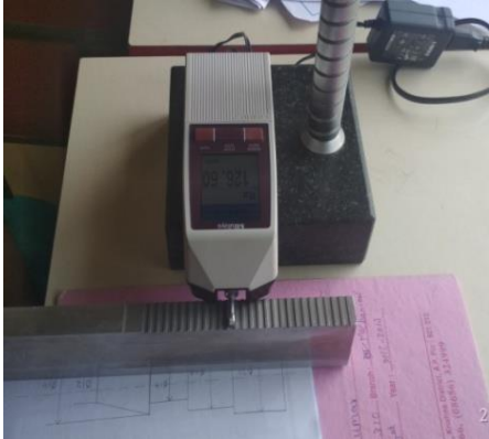
Figure 7 R_a measurement by using surface roughness tester
