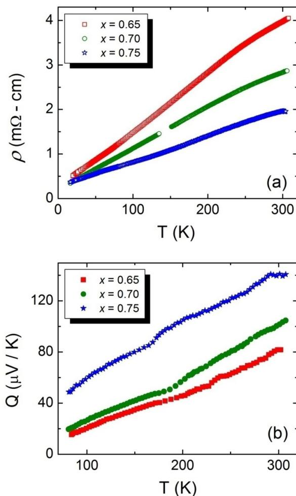
**Figure. 2 – Temperature dependence of (a) electrical resistivity ( $\rho$ ) and (b) thermoelectric power ( $Q$ ) of  $\text{Na}_x\text{CoO}_2$  with  $x = 0.65, 0.7$  and  $0.75$ .**
