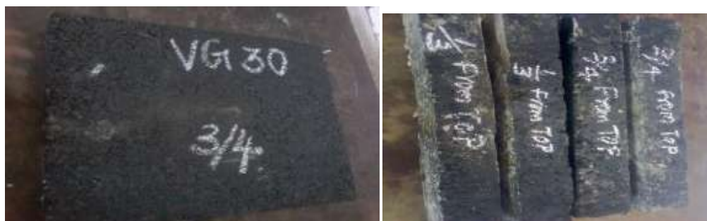
Fig 8. Images of Fatigue test beams
