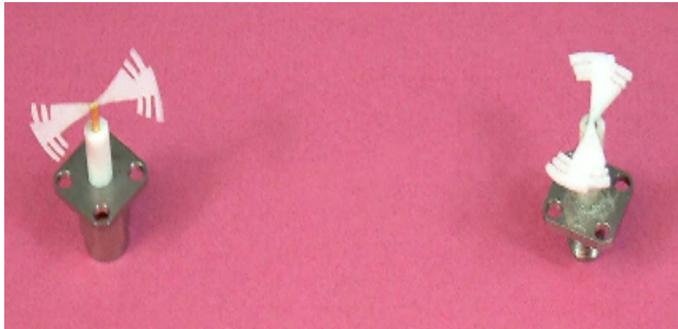
Figure 5.1(a) Dielectric log- periodic antenna
