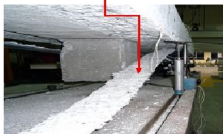
Figure 7: Failure mode of beam B7
