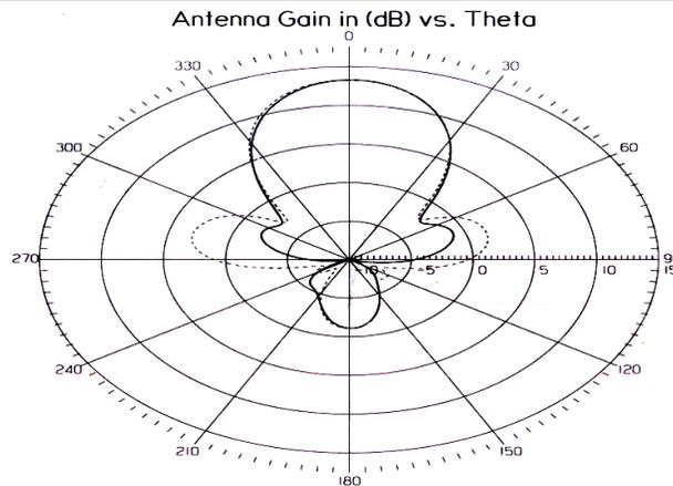
**Figure 18: Radiation pattern for antenna 2. at —  $\Phi = 45^\circ$  and - -  $\Phi = 90^\circ$  at resonance frequency**
