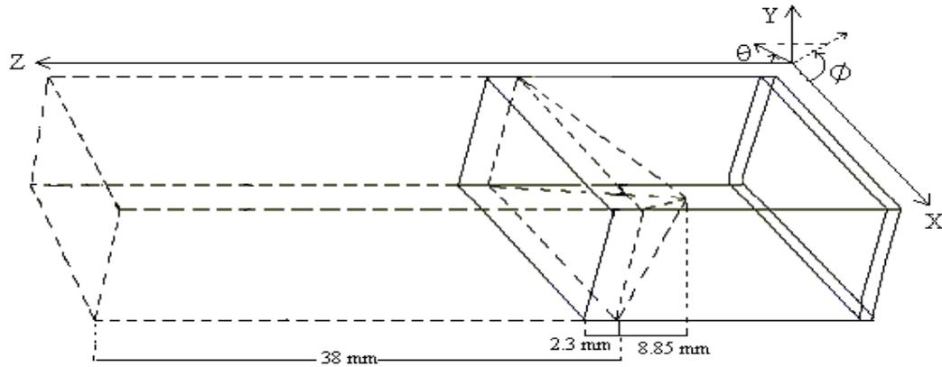
**Figure 11. Dielectric slab antenna with pyramidal matching section**
