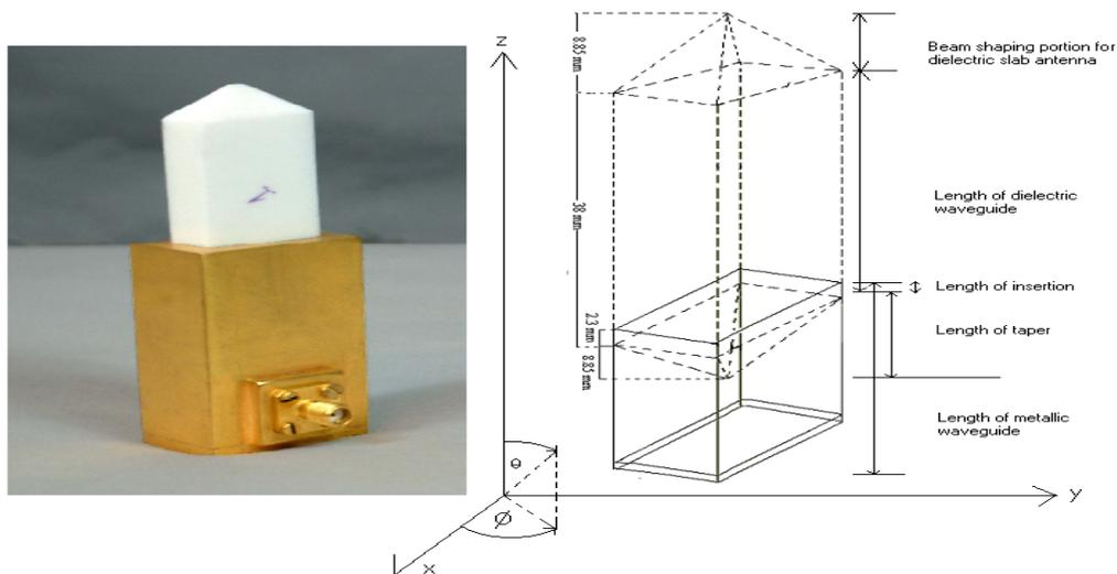
**Figure 2: Dielectric Slab antenna with pyramidal matching section**
