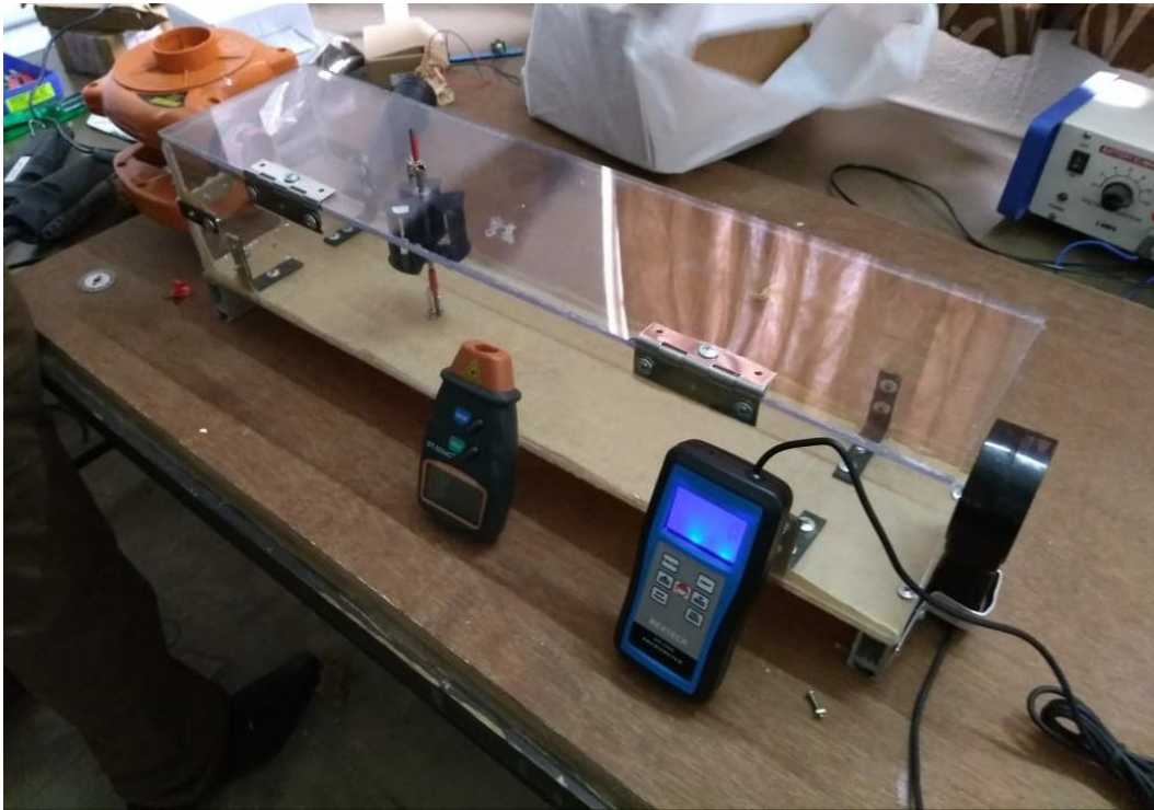
Fig. 5: Testing of Micro-Darrius vertical axis wind turbin
