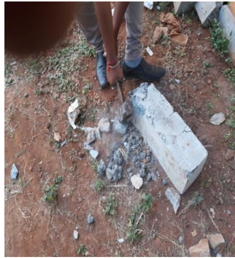
Fig 2: Separation Of RCA From Cubes
