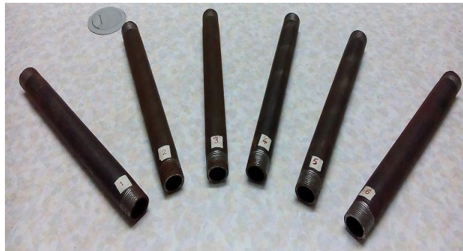
Figure 7. Seamless pipe-pieces (Length: 305 mm, Diameter: 30 mm) as CUT
